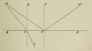
are shown that if a ray proceed from a point O within a piece of glass to a point C at its surface A B, and if O C b at its incidence be less than 41° 49′, it will be refracted in some
